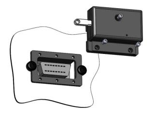
Plug in the lock and fix it with the provided M3 screws
